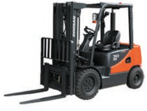
4-wheel, LPG/Diesel pneumatic tire 3,000 - 36,000 lb capacity
