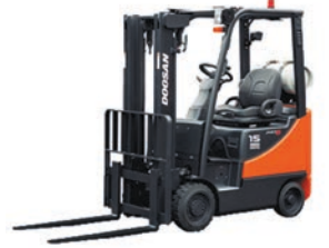
4-wheel, LPG cushion tire 3,000 - 6,500 lb capacity
