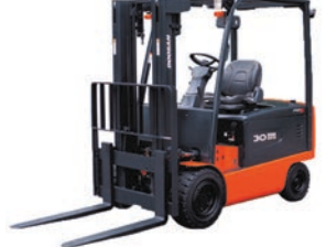
4-wheel, Electric cushion tire 3,000 - 6,500 lb capacity
